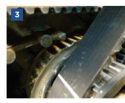
**Adjust clearance** between **exhaust and intake valves** of cylinder 1, intake of cylinder 2 and exhaust of cylinder 3, which in this point are fully raised, such as in the picture below:
