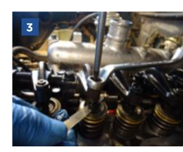
Once all clearances have been adjusted, **turn the crankshaft 360° clockwise** (to match the mark of the crankshaft pulley; the camshaft pulley will not match since it has only turned 180°), then adjust exhaust and intake valves of cylinder 4, exhaust of cylinder 2 and intake of cylinder 3 as in the previous step:
